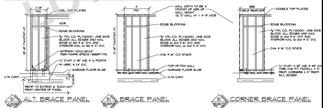
FOR ALTERNATE BRACE PANEL USE ON FRONT OF GARAGE, FOUNDATION FOOTING MUST RUN CONTINUOUSLY ACROSS THE GARAGE DOOR OPENING
